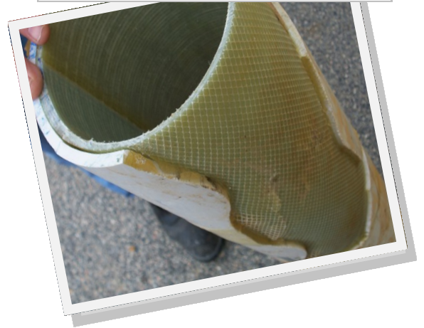
Below: Original pipe cracked but IRSI Point Repair remained intact.
